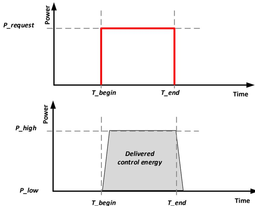
Fig. 6. Baseline method for calculating the delivered control energy. The y-axis depicts the consumed power for a load or delivered power for a generator.  $T_{begin}$  indicates the beginning of the control energy activation and  $T_{end}$  indicates the end of the control energy activation.  $P_{request}$  is the requested control power.  $P_{low}$  is the power of the technical unit before control energy activation and  $P_{high}$  is the power after the control energy activation.
