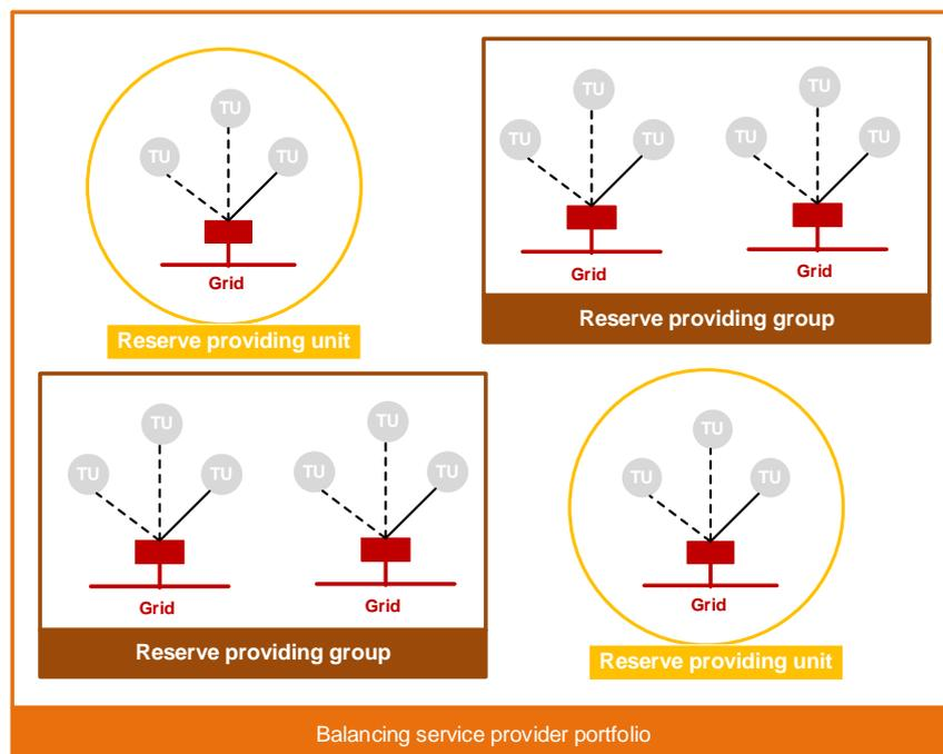
Fig. 3. Example of a BSP portfolio with two *reserve providing units* and two *reserve providing groups*. A *reserve providing group* can also include *reserve providing units*. A *technical unit* (TU) can either be a power generating module or a demand unit. The red box depicts a grid connection point.
